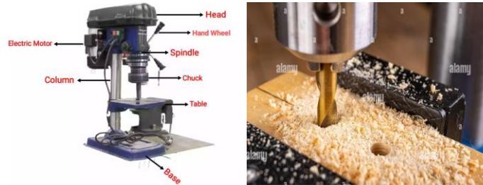
Pillar drills are free standing machine tools used by engineers that use high powered motors to rotate drill bits at varying speed.
