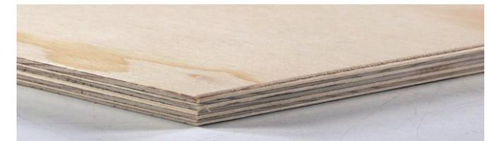
Sheet materials manufactured from layers or particles of wood. Reddish brown or white in colour. Layered in odd numbered sheets. Strong. Susceptible to splintering Used in sheds and cladding, furniture, flooring, boats (marine ply).
