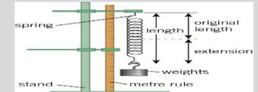
6. If too much force is added, then a spring does not return to its original shape. The spring has reached its elastic limit.
